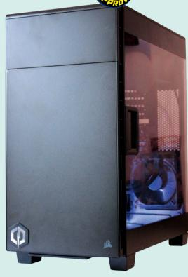
600C's airflow helps in this respect. The other key area where the two machines differ is CPU cooling - the CyberPower has a single-fan 120mm Corsair H55 cooler, compared with the two-fan, 240mm Corsair H100i cooler in the PC Specialist, although the latter is arguably overkill for a Core i5-6600K chip.
