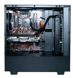
The graphics card and motherboard are both made by MSI. As the name suggests, the Z<sub>3</sub>70-A Pro isn't a specialist gaming board, but it does have one showy flourish - a jagged lighting strip on the left side. Cyberpower also includes two programmable strips of RGB LEDs. With all these darkcoloured components, though, I'd lean towards a tasteful white illumination rather than anything too colourful.
